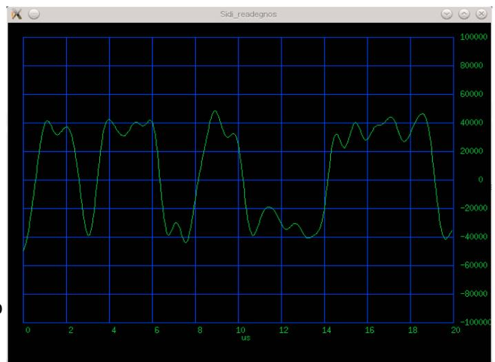
Fig 4. Directly demodulated spread code
