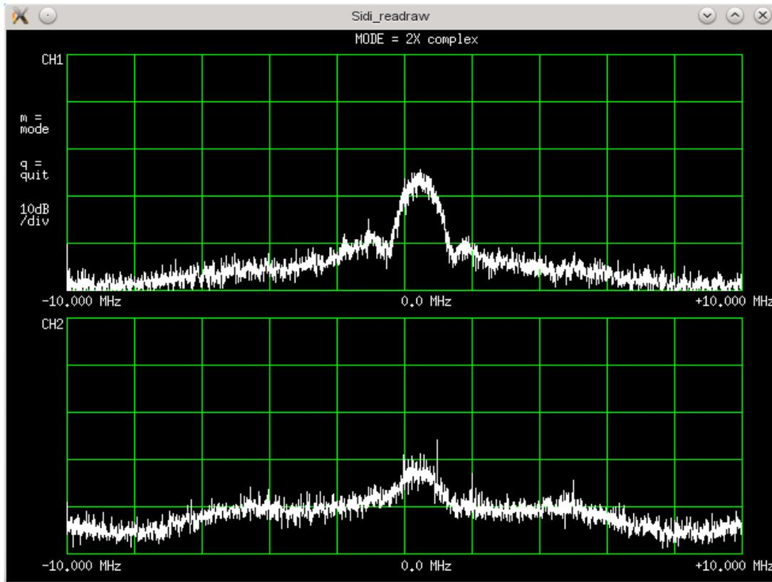
Fig 3. EGNOS signal from 15W (Inmarsat AOR), top: 3m dish, bottom: 6 turn helix
