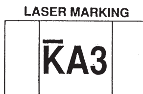
Example shown is a 1,000 pF capacitor.
