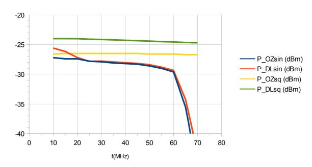
Comparison of the results shows the difference in displayed power (dBm) when the input signal is sine wave and different from sine wave (square).
