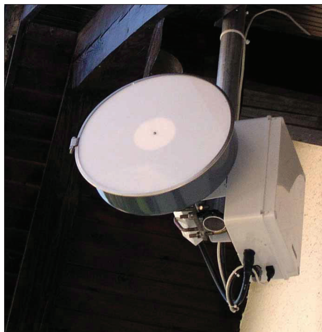
Slika 4 - Predelan 50Mbps link - WLAN bridge
