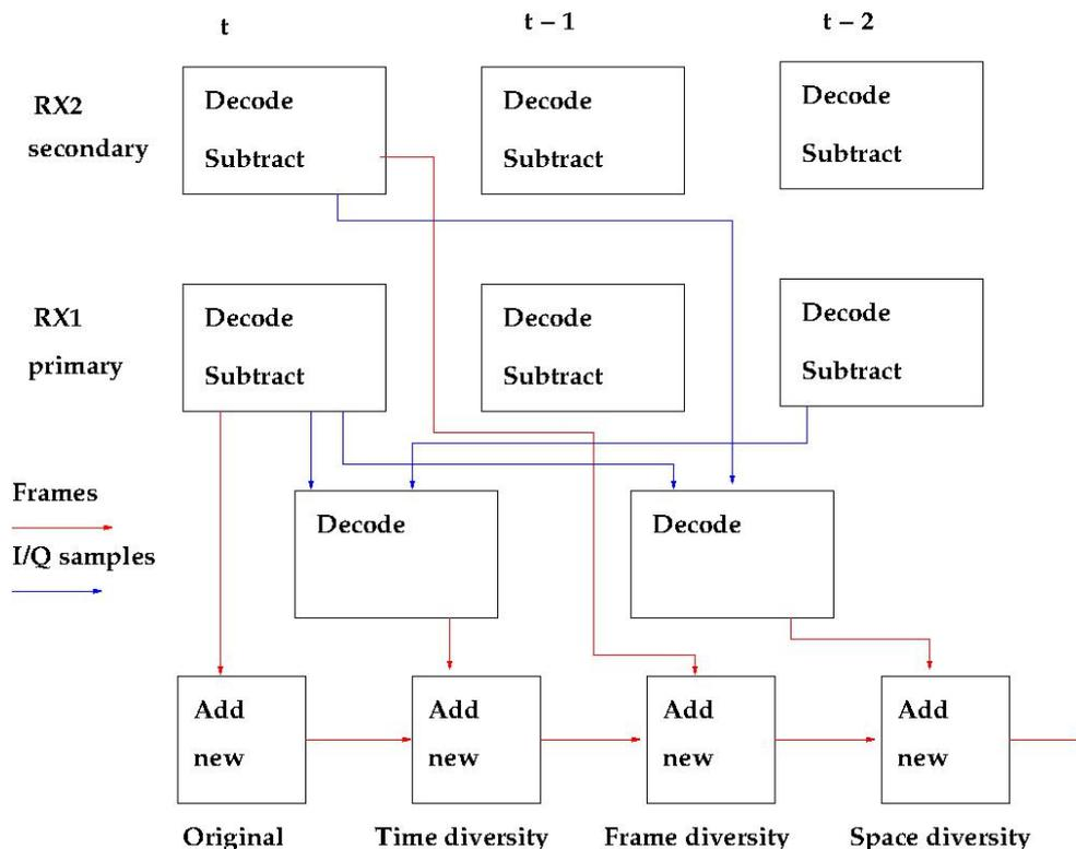
Data flow in WSJTX with diversity. Temporary file is exchanged with decoded frames and residual audio sample.
