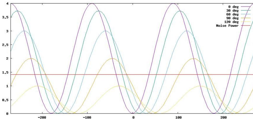
Power of two shifted tones:  $(\sin(\omega t) + \sin(\omega t - \phi))^2$  for different phase difference  $\phi$ . Summing up power of two uncorrelated noise sources results in 1.4 times increase in noise power.
