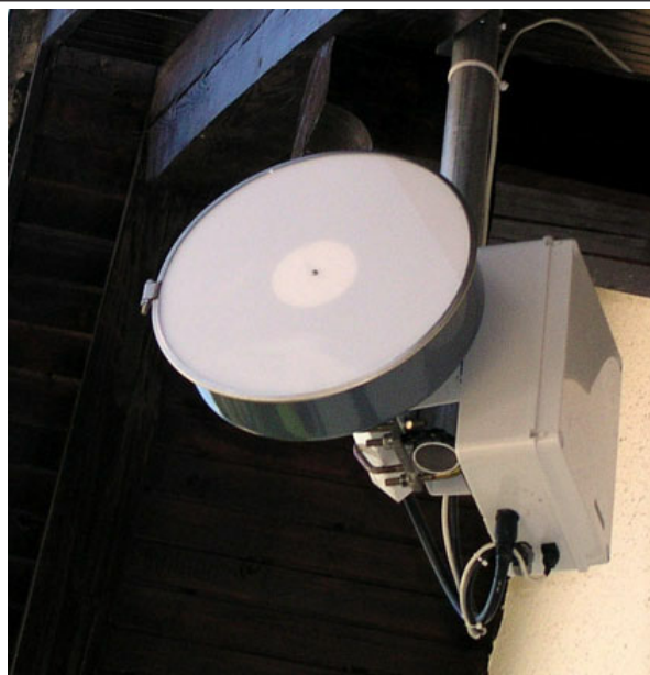
Slika 2.2 - Predelan 50Mbps link, WLAN bridge
