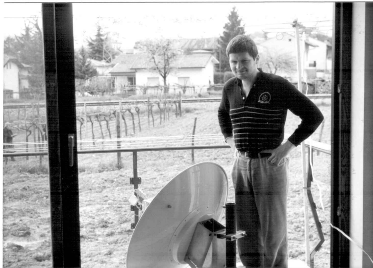
Fig. 1. - The 90 cm diameter dish pointed to Intelsat \bar{V} A at 27.5^\circ W.
