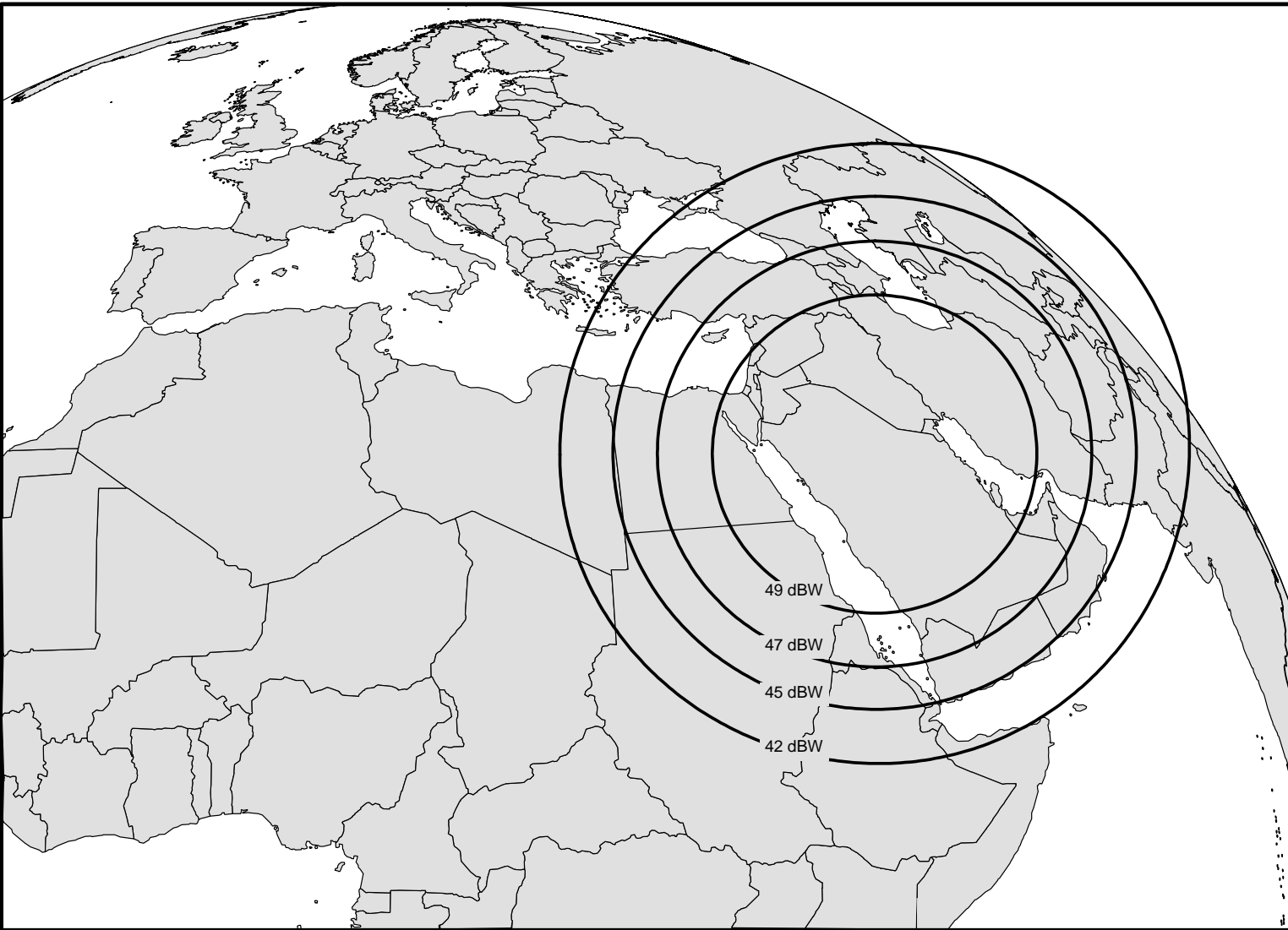
Figure 5 : Example of Steerable Beam Coverage (HOT BIRD™ 3, 4)
