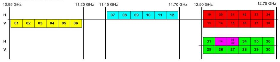
Figure 1. Hellas SAT frequency Plan
