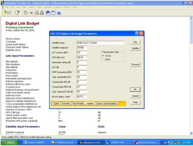
G/T and EIRP can be extracted from the coverages provided in Annex C G/T<sub>Athens</sub>=6.6dB/K EIRP<sub>London</sub>=53dBW
