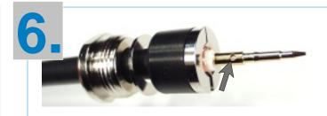
Slide center pin cautiously on center conductor and solder carefully through the little hole..
